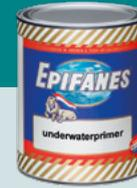
A bituminous primer reinforced with aluminum providing a tough impermeable film. For the underwaterprotection of wood steel or aluminum. For touch ups or full treatment prior to the application of antifouling paints. May be overcoated with most types of antifouling. We recommend to first make a test patch to check the solvent resistance of the Epifanes Underwaterprimer. Antifouling should be applied in full layers without repeated striking.
