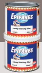
A strong two-component finishing filler based on epoxy resins. Very fine and shrink free. Provides a very smooth surface. Apply in thin layers only (max. 1 mm.). Prior to use, stir each component separately and then thoroughly together until color is uniform. Do not use under 12°C. (60°F). Best sandable properties are between 24 and 48 hours.
