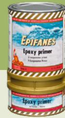
An anti-corrosive primer based on an epoxy resin and zinc phosphate as the anti-rust agent. High build, high filling capacity and easy sanding. For use as a filling primer in a two-component paint system on (ply-)wood and fiberglass and as an anti-corrosion primer in a two-component paint system on steel and aluminum. For optimum adhesion always thin first coat on bare plywood and metal by 20-25% and apply by stiff brush.
