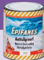
A one-component, semi-gloss, urethane/alkyd based nonskid deckpaint containing measured amount of polypropylene beads as the nonskid agent. To avoid the intake of moisture, apply Nonskid Deckcoating on at least 2 high gloss coats. Application by shorthaired fur roller provides an even distribution of the beads. Stir well before and during use. Allow the final coat at least 72 hours to harden thoroughly.
